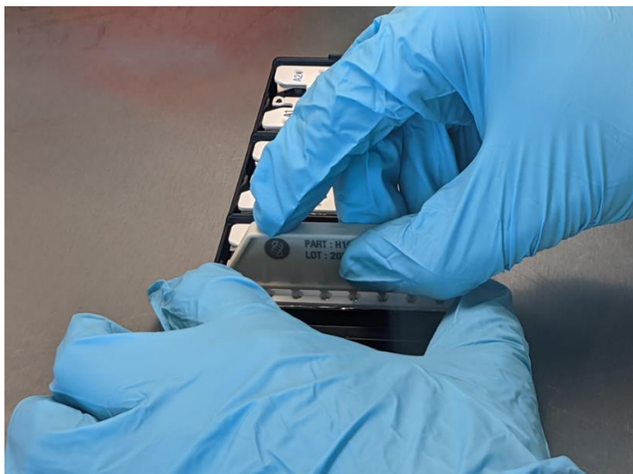
Figure 6: Hold the chip with one hand and your Piercing Tool with the other.
