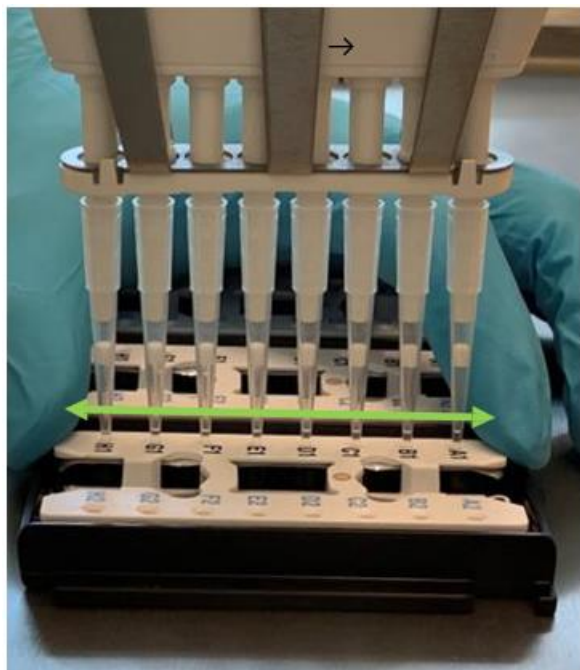
Figure 4: Correct positioning of an 8-channel pipette for sample injection
