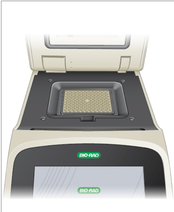
图 9: PTC Tempo 96、PTC Tempo 384、PTC Tempo Deepwell、PTC Harmony 96 和 PTC Harmony Deepwell 样品反应模块和热盖
