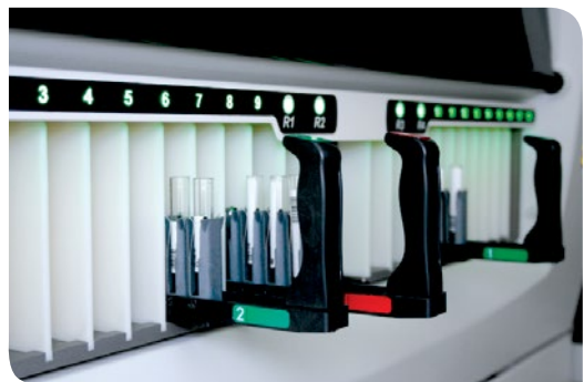
Loading area for up to 180 samples and 28 reagent vials
