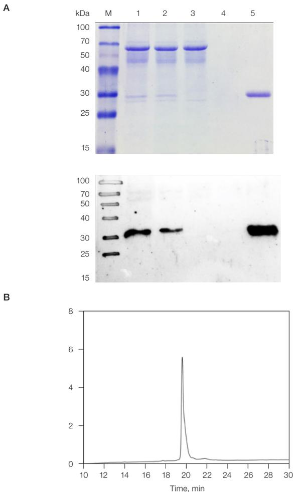
**Fig. 1.** Analysis of fractions collected during the Nuvia IMAC Resin purification process of His6-tagged receptor binding domain (rRBD). **A**, SDS-PAGE and western blot analysis of anti-S antibody fractions under reducing conditions. M, protein marker; 1, Sf9 cell expression supernatant; 2, diafiltered sample; 3, flow-through; 4, washing step; 5, IMAC elution fraction. **B**, RP-HPLC analysis of rRBD purified by Nuvia IMAC Resin.
