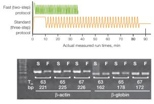
Fast two-step protocol results are comparable to those generated using standard protocols.  $\beta$ -actin and  $\beta$ -globin targets were amplified from human genomic DNA using iTaq DNA Polymerase. Standard (S) protocol, 1.5 hr; fast (F) protocol, 35 min.
