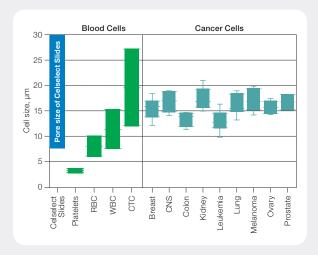
Pore size of Celselect Slides is suitable for diverse cell capture. CNS, central nervous system; CTC, circulating tumor cells; RBC, red blood cells; WBC, white blood cells.
