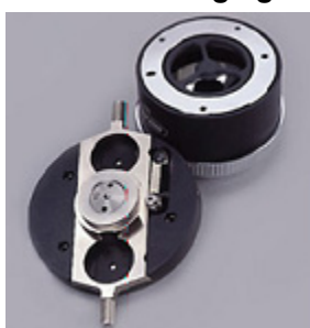
Figure 5. Varian micro slide on ATR accessory
