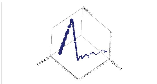
Fig. 3. Reaction pathway in terms of the PCA scores. Time in the reaction sequence shown by increasing point size.
