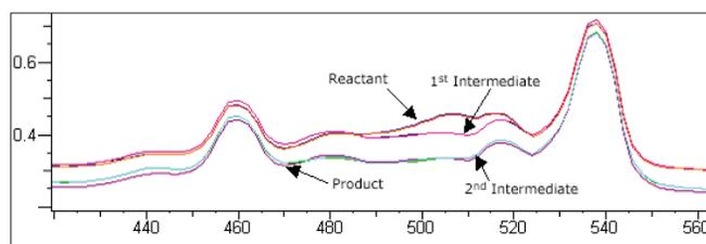
**Fig. 5.** Magnified spectra at the nodes of the reaction trajectory.
