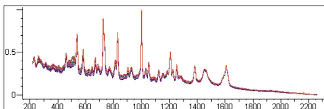
Fig. 1. Normalized Raman spectra of a batch process throughout the reaction time.
