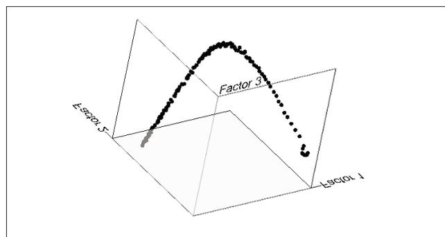
Fig. 2. A reaction curve for the pharmaceutical process, in the PCA scores plot.
