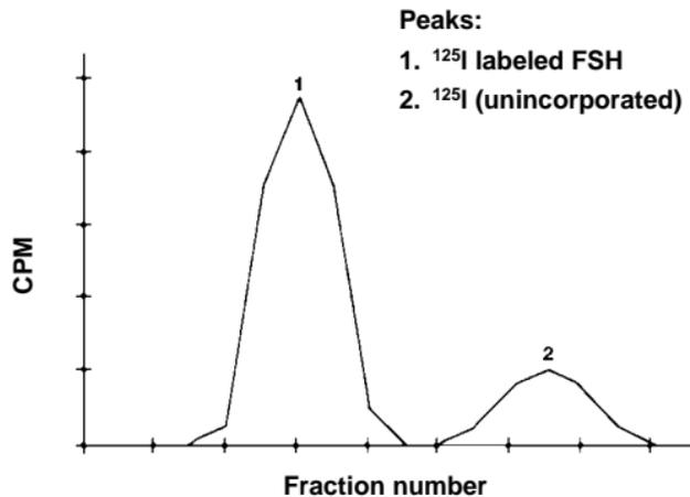
**Fig. 5.2. Separation of radiolabeled protein from unincorporated radiolabel.**
