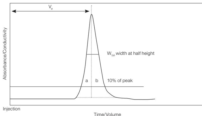
Fig. 1. A simulated chromatogram illustrating the calculation of HETP, rHETP, and  $A_s$  values.
