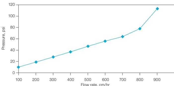
**Fig. 3. Pressure flow curve of Nuvia IMAC Resin packed in a Vantage L Column (1.6 x 20 cm) column at a CF of 1.28.**
