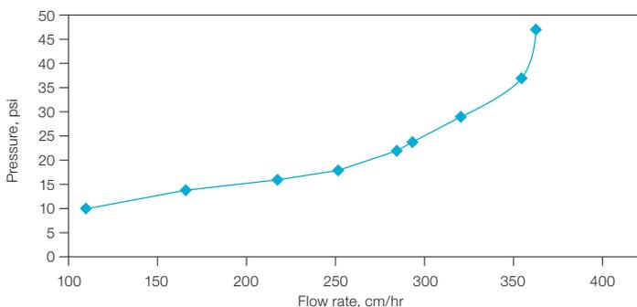
Fig. 5. Pressure flow curve of Nuvia IMAC Resin packed in an InPlace Column (20 x 20 cm) at a CF of 1.2.
