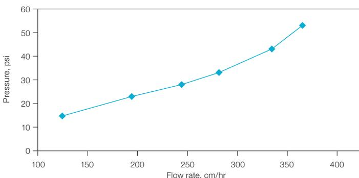
Fig. 4. Pressure flow curve of Nuvia IMAC Resin packed in a BPG 100/500 Column (10 x 20 cm) at a CF of 1.29.
