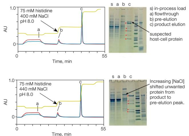
**Fig. 3. Chromatograms and gels from anion exchange process development experiments.** OD 260 (—); OD 280 (—); conductivity (—). \* Proteins presumed to be virus capsid components. AU, absorbance units.
