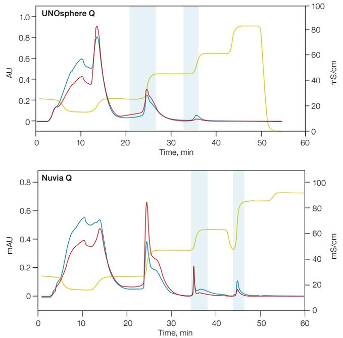
**Fig. 2. Behavior of the crude harvest on the UNOsphere Q and Nuvia Q Columns.** OD 260 (—); OD 280 (—); conductivity (—). Blue shading indicates detection of significant transgene expression. AU, absorbance units.
