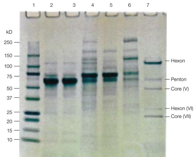
**Fig. 6. SDS-PAGE of intermediates and the final product.** Lane 1, MW marker; lane 2, Nuvia cPrime load; lane 3, Nuvia cPrime flowthrough; lane 4, Nuvia cPrime elution/Nuvia Q load; lane 5, Nuvia Q flowthrough; lane 6, Nuvia Q pre-elution; lane 7, Nuvia Q product.
