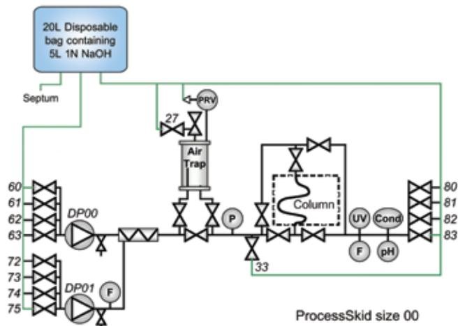
**Fig 2. Schematic of Bio-Rad process chromatography skid 00.**
