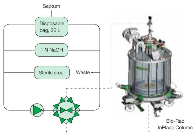
Fig. 2. Hardware installation for the bacterial challenge test.
