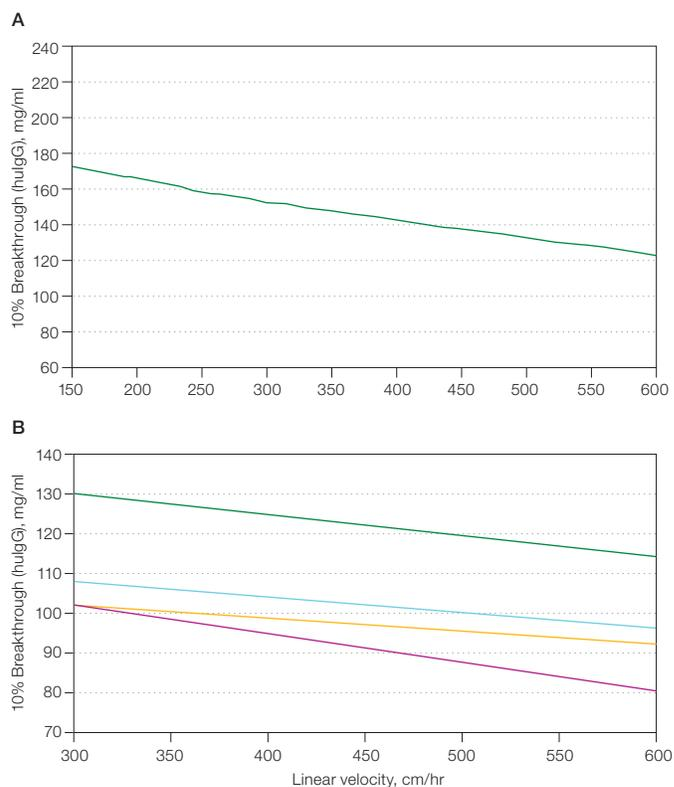
**Fig. 1. Binding of hulG by Nuvia S media at various linear velocities.** **A**, binding on a Nuvia S column (1.1 x 20 cm). **B**, comparison of Nuvia S with commercially available CEX media. (—), Nuvia S; (—), CEX 1; (—), CEX 2; (—), CEX 3. Column size, 1.1 x 9.5 ± 0.3 cm.
