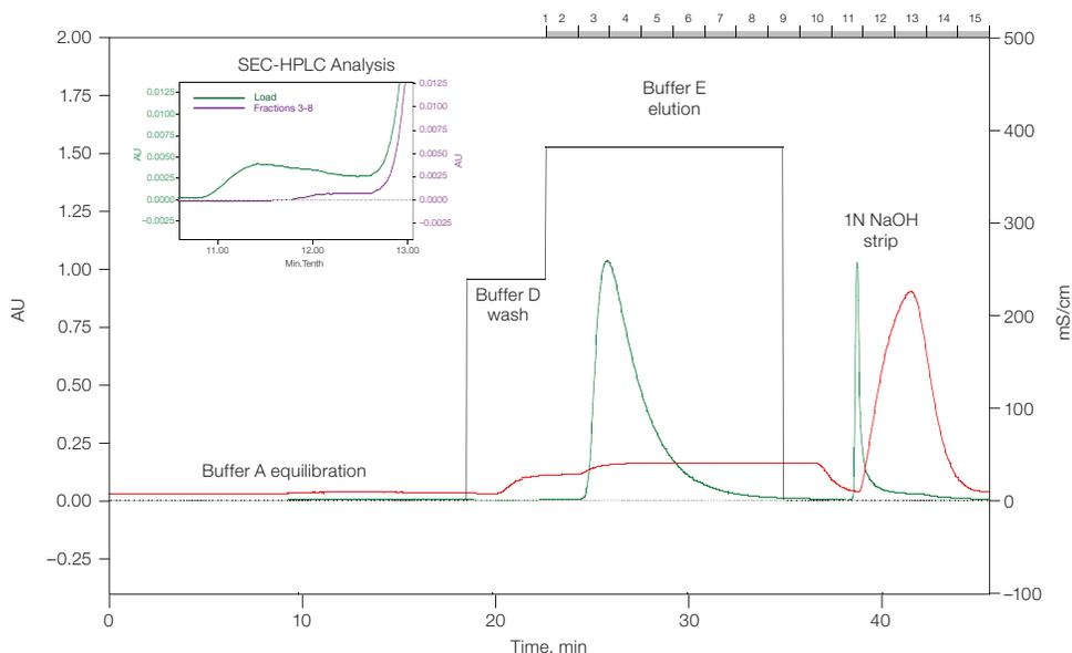
**Fig. 4. Intermediate polishing of mAbG by Nuvia S media: Removal of mAbG aggregates.** Both loaded material and pooled eluate fractions were analyzed by SEC-HPLC to assess the contamination level of mAbG aggregates. (—), OD<sub>280</sub>; (—), conductivity; (—), salt steps.
