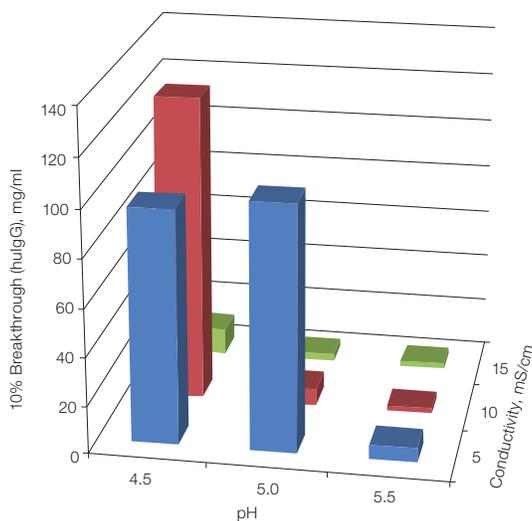
**Fig. 2. Dynamic binding capacity of hulG by Nuvia S media as a function of load, pH, and conductivity.** Nuvia S was packed into 0.7 x 5.5 cm columns and equilibrated with the appropriate binding buffer. HulG was loaded in the same buffer at a flow rate of 300 cm/hr.
