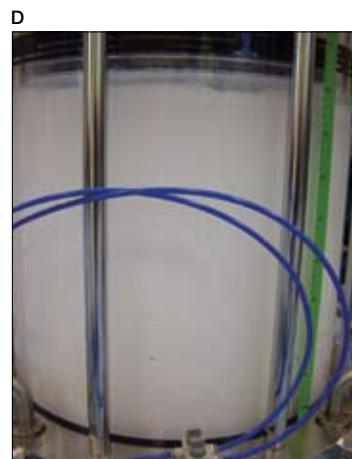
Fig. 3. Bio-Rad InPlace column repacking. A , initiation of upflow at 100 cm/hr while the top piston was raised; B , end of upflow and bed resuspension in PBS at 40% (v/v); C , fully resuspended bed; D , sparging with air was performed for >10 min to bring the suspension to homogeneity while preventing shearing of CHT.
