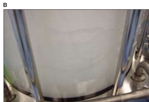
Fig. 2. Fully packed 45 cm Bio-Rad InPlace column. CHT Type I support, 40 \mu\text{m} , was hydrated and packed in a 40% (v/v) suspension in PBS.
