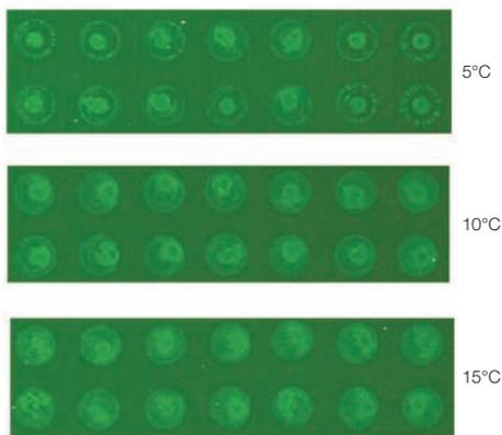
**Fig. 3. Temperature dependence of protein immobilization.** Fluorescence images show dip-coated glass slides printed with 75  $\mu\text{g/ml}$  BSA-FITC in PBS, pH 5, at 65% RH. Three different temperatures are shown.
