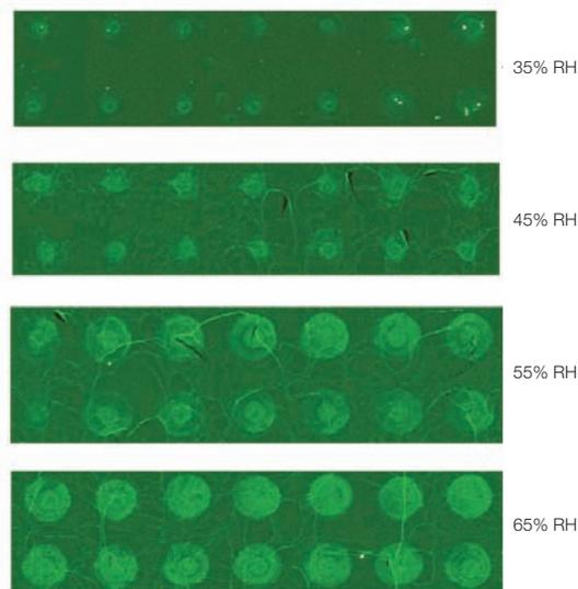
**Fig. 4. The effect of RH on protein immobilization.** Fluorescence images show 75  $\mu\text{g/ml}$  BSA-FITC printed onto a dip-coated glass slide at 10°C and pH 5. Four different RH levels are shown.
