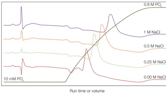
**Fig. 5. Elution of sheared salmon sperm DNA from CHT ceramic hydroxyapatite.** Data compare the behavior of DNA on CHT as a function of sodium chloride concentration. Increased NaCl concentration improved DNA retention.
