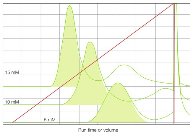
**Fig. 3. Elution of protein A-purified IgG1 from CHT ceramic hydroxyapatite.** A 40 column volume linear gradient to 1.0 M NaCl (—) at three constant phosphate concentrations is shown. Data indicate a trend of decreasing aggregate resolution with increasing phosphate concentration.
