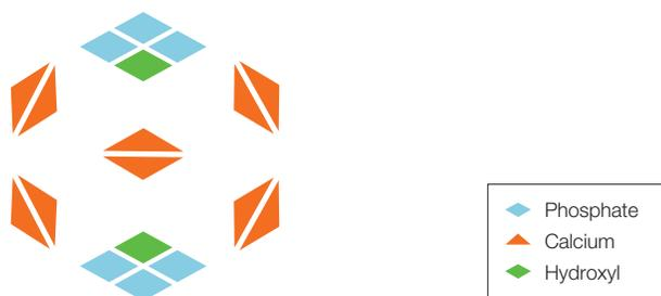
**Fig. 1. Crystal structure of CHT ceramic hydroxyapatite,  $\text{Ca}_{10}(\text{PO}_4)_6(\text{OH})_2$ .** Each molecule consists of five positively charged calcium pairs (C-sites); two phosphate triplets (P-sites), each with six negatively charged oxygen atoms; and two hydroxyl residues.
