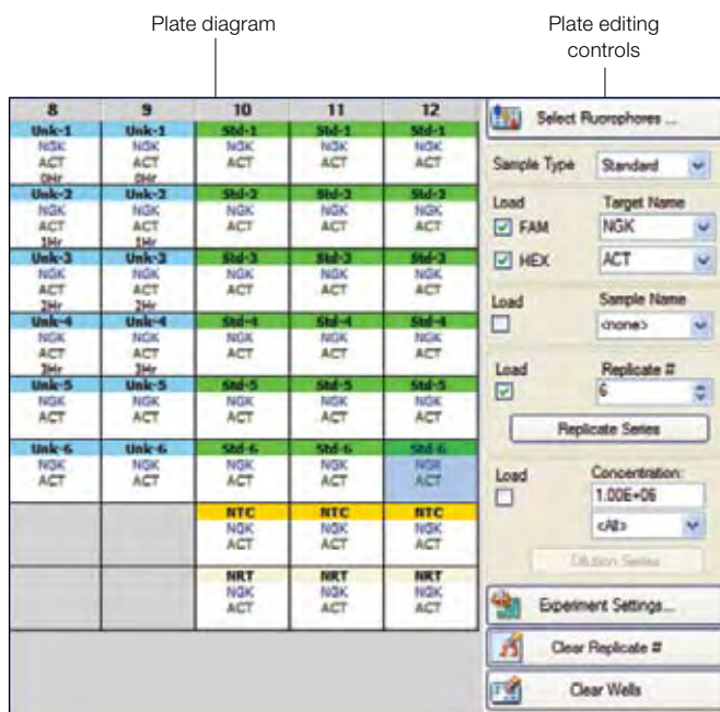
Fig. 2. Plate Editor. In the plate diagram, select the wells you want to load. Use the plate editing controls to enter or edit well contents.
