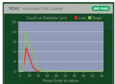
Fig. 15. Histogram for live and dead cell count (sample with trypan blue dye).
