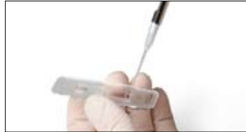
Fig. 7. Loading the TC10 counting slide.
