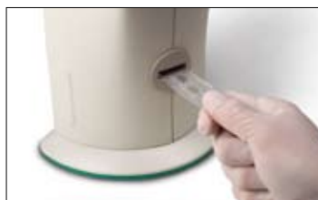
Fig. 9. Inserting the TC10 slide into the TC10 cell counter.
