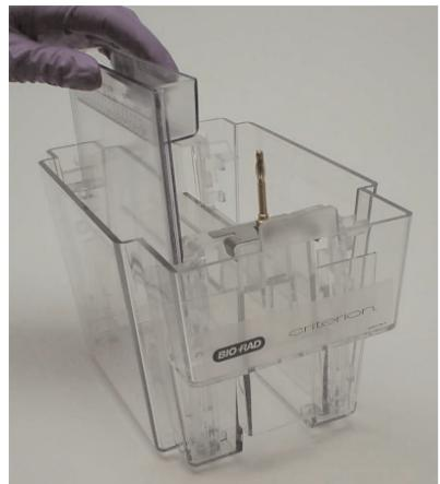
8. Place the lid on the tank, aligning the color-coded banana plugs and jacks. See section 3.6 for power conditions.
