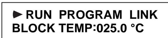
The current block temperature is always displayed at the main menu. The right/left arrow keys may be used to choose **RUN**, **PROGRAM**, or **LINK**. **RUN** is the default choice. Section 3 explains in detail how to create, edit, link, and run programs.
