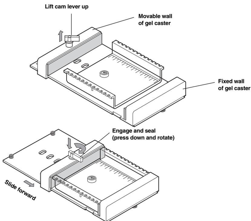
Fig. 2.1. Sealing the UVTP tray for gel casting.
