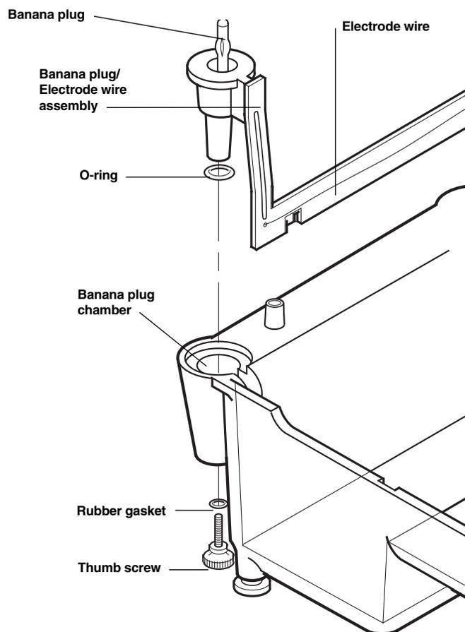
Fig. 4.1. Removal of banana plug/electrode wire assembly.
