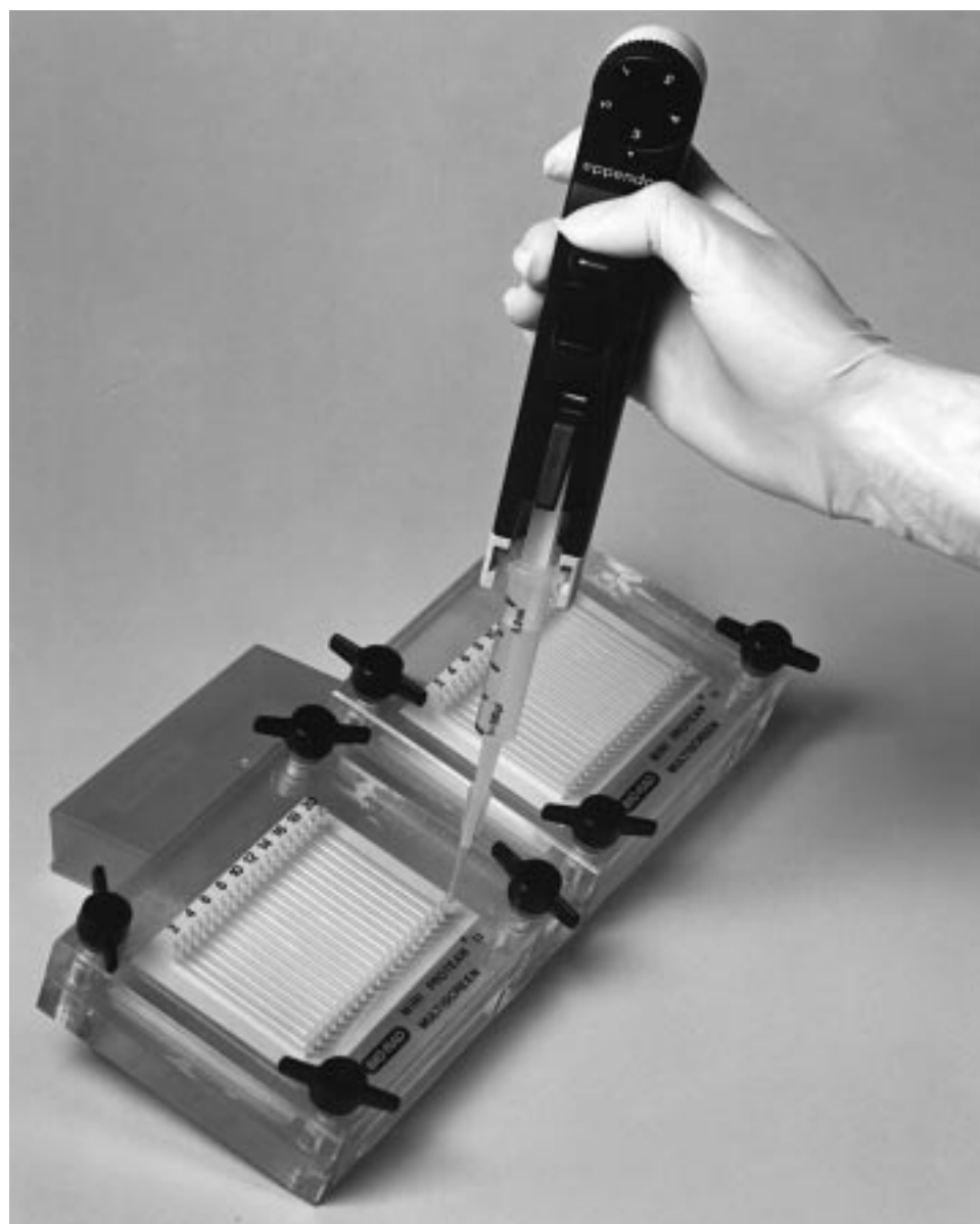
Fig. 3. Tilt the multiscreen apparatus toward you during sample application.
