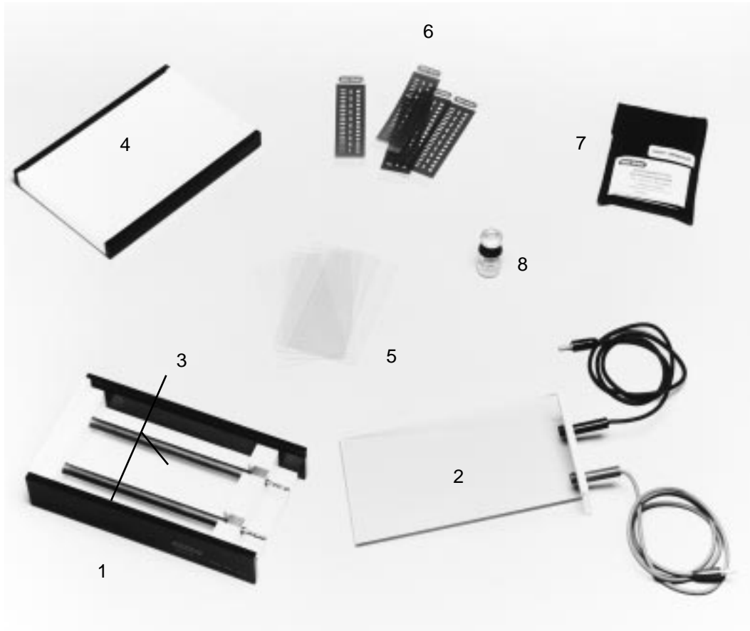
Fig. 1.1. Model 111 Mini IEF Cell. Outer chamber (1), sliding, interlocking lid with power cables (2), graphite electrodes (3), casting tray (4), glass plates (5), sample templates (6), gel support film (7), and 5 ml Bio-Lyte 3/10 ampholyte (8).
