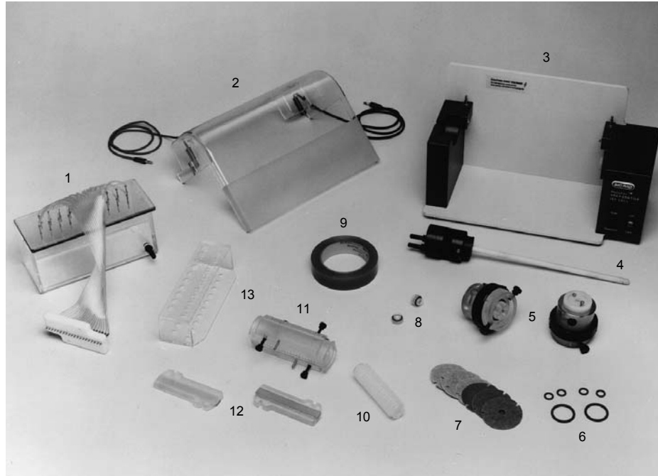
Fig. 2.1. Rotofor components. Harvesting apparatus (1), safety cover (2), housing (3), cooling finger (4), electrode assemblies (5), O-rings (6), ion exchange membranes (7), vent buttons (8), sealing tape (9), membrane core (10), focusing chamber (11), cell covers (12), test tube rack (13).
