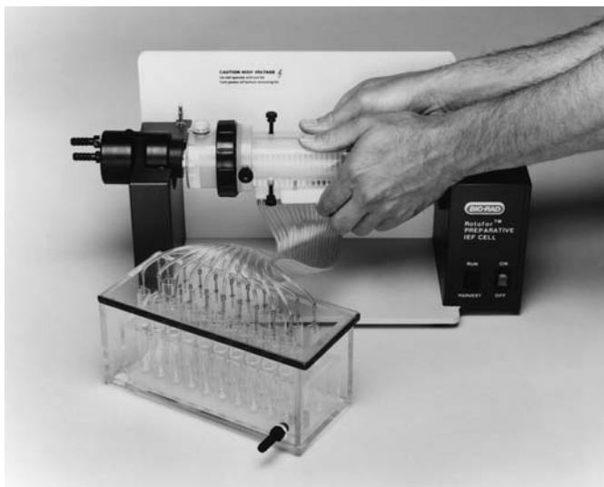
Fig. 4.2. Harvesting samples after focusing is complete. Make sure thumbs do not cover the uppermost ports.
