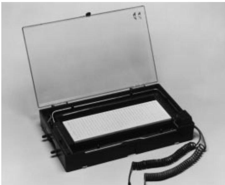
The versatile Bio-Phoresis horizontal electrophoresis cell accommodates interchangeable accessories which allow you to perform immunoelectrophoresis, electrophoresis, and electrofocusing in the same cell. Only the addition of the appropriate electrodes, a power supply, and an applications kit for the specific technique is required.
