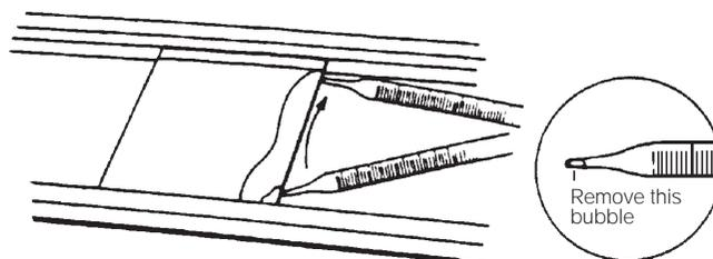
a). Clear bubble from end of pipet. b). Start solution at one corner of plate and move it along the edge to form a front. Be sure the solution contacts both the plate and tray. Avoid trapping air bubbles by releasing the solution slowly.
