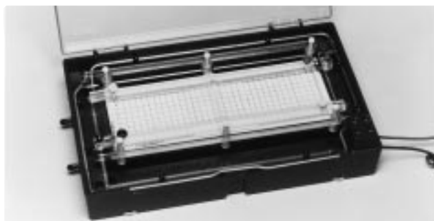
B. Posiforce electrode holder assembled with 360 mm electrodes.
