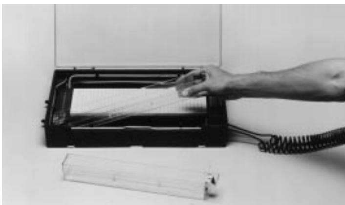
5. Install the electrode/buffer chambers. Place the electrode/buffer chambers in the cell alongside the cooling platform. Locate the chamber with the colored dot (red or black) which corresponds with the colored dot (red or black) on the cell. This will insure that the anode and cathode connections are correct. The electrical connections are at opposite ends to equalize the electrical field.
