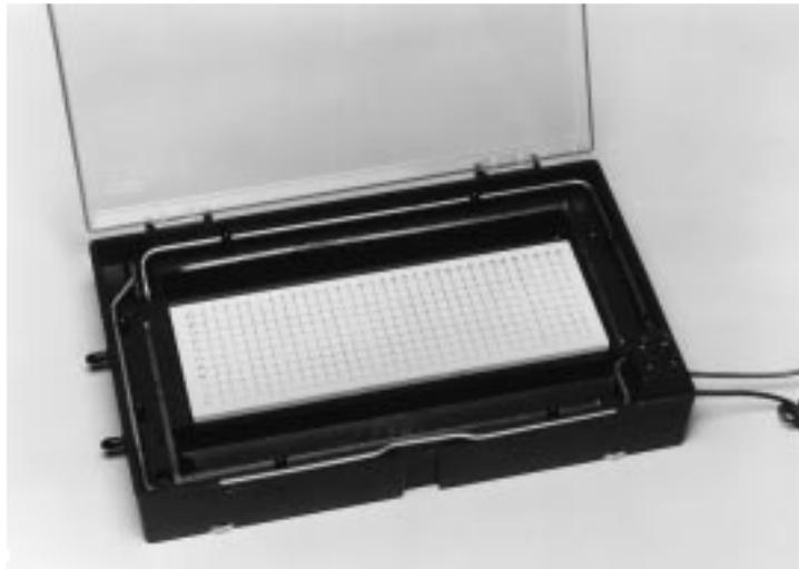
1. Connect 1/4" tubing from the water source (tap water line or the outlet port of a refrigerated water bath) to the inlet port of the cell.
