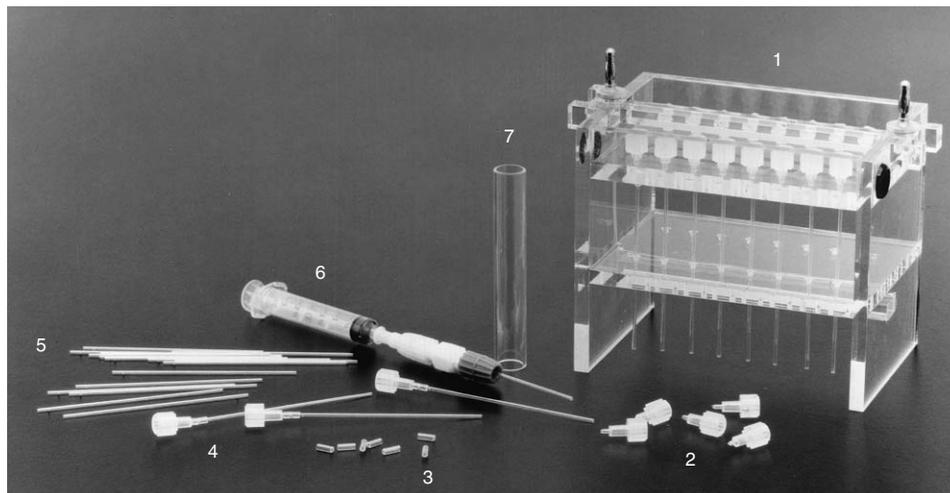
**Mini-PROTEAN tube cell (catalog # 165-2961).** Includes tube cell module (1), sample reservoirs (2), capillary tube connectors (3), tube setup; sample reservoirs/capillary tube connector/capillary tube (4), capillary tubes (5), tube gel ejector (6), and casting tube (7).
