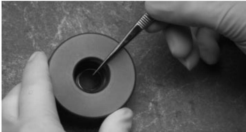
**Fig. 4.7. Rupture disk insertion into recess of retaining cap.**
