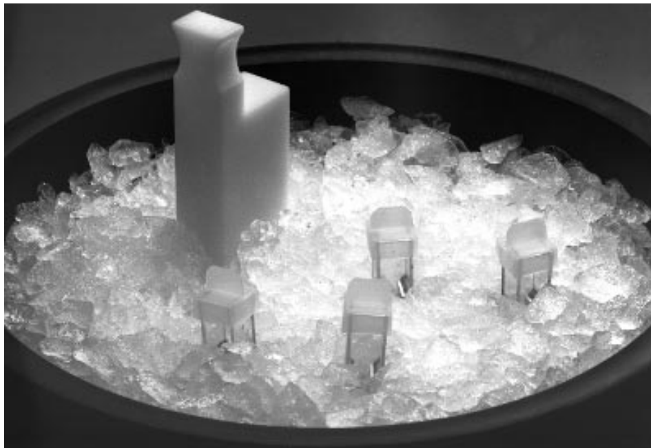
Fig. 7. White cuvette slide and cuvettes equilibrating to 0 °C before the pulse.
