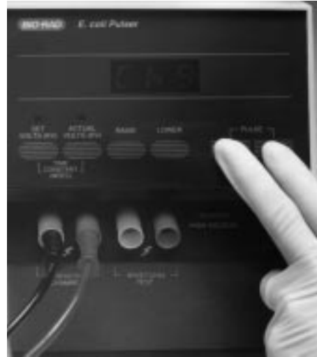
Fig. 5. A display of “Chg” indicates that the capacitor is being charged.
