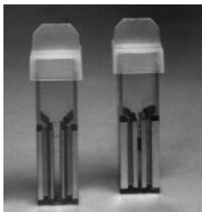
Fig. 2. 0.2 cm and 0.1 cm electrode gap cuvettes.
