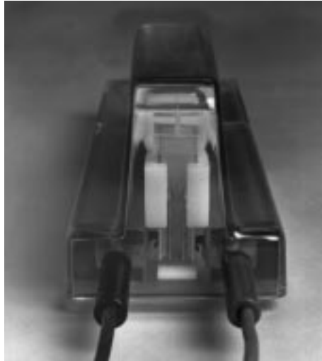
Fig. 4. The slide with a cuvette at the back of the shocking chamber.
