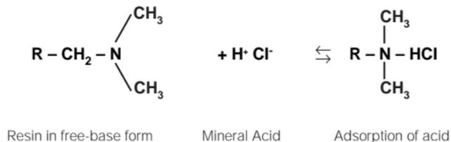
**Fig. 1. Adsorption of hydrochloric acid.**
