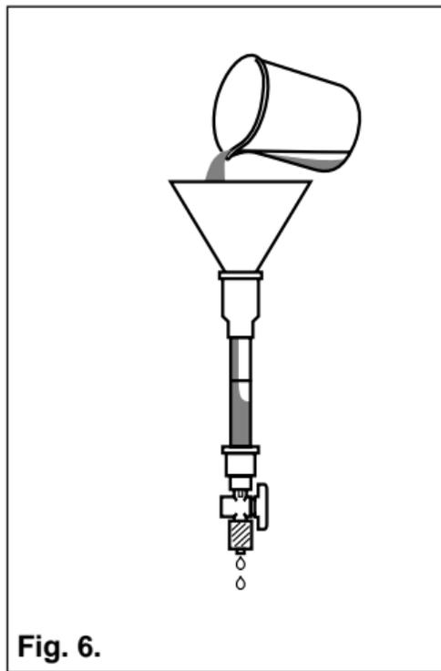
6. Pour the even slurry into the column in a single, smooth movement. Avoid splashing the slurry, to insure even packing, and to avoid trapping air bubbles (Figure 6).
