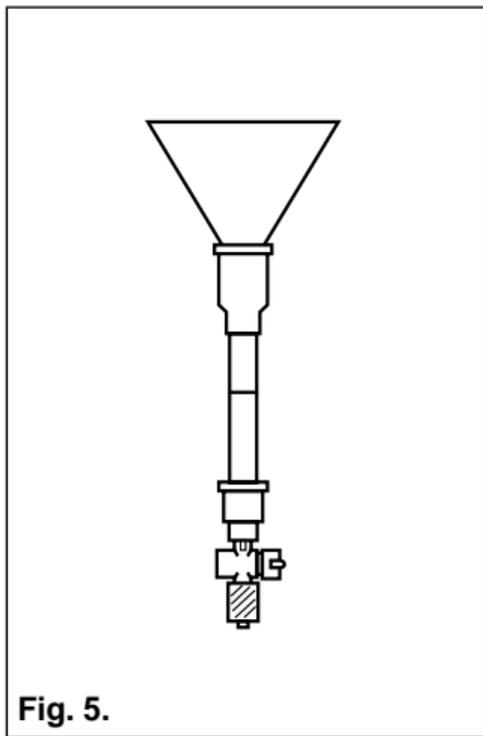
5. Affix a funnel to top of column, close column exit, and add enough buffer to fill 20% of column (Figure 5).
