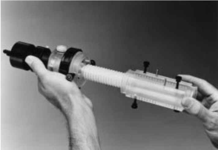
Fig. 4. Slide the focusing chamber over the membrane core.
