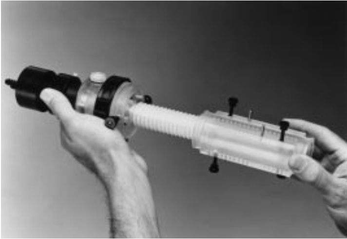
Fig. 4. Slide the focusing chamber over the membrane core.
