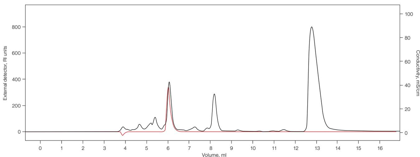
**Fig. 6. ChromLab Software evaluation of RI detector data.** Overlay chromatograms of a reference fructose solution (—) and secondary fermentation wine sample (—).
