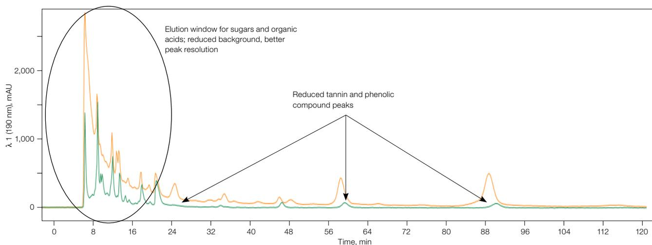
**Fig. 2. Treatment of a sample with activated charcoal to remove background interference.** Comparison of an untreated wine sample (—) and the sample treated with activated charcoal (—) at 190 nm.
