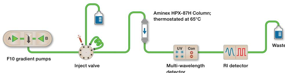
Fig. 1. Schematic of the NGC Quest System, Aminex Column with column heater, and UV multi-wavelength and RI detectors in series.
