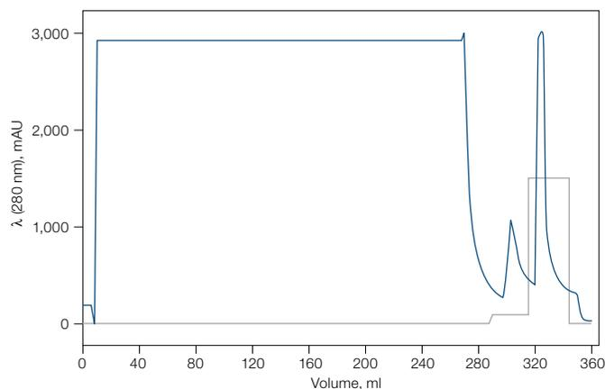
**Fig. 1. PPARγ-LBD purification using 5 ml Nuvia IMAC on Bio-Rad NGC Quest system plus sample pump.** Using the sample pump, 240 ml of clarified lysate was loaded onto a 5 ml Nuvia IMAC column. The protein was eluted with a 50% buffer B after a 3% buffer B wash to remove weakly binding contaminants. λ (280 nm) (—); %B (—).
