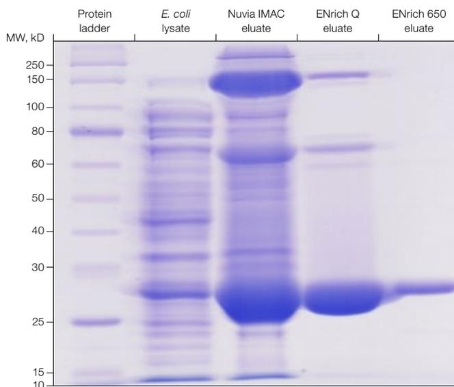
**Fig. 4. SDS-PAGE of the PPAR $\gamma$ -LBD purification workflow.** Approximately 10  $\mu$ l of the pooled fraction after each step was run on an SDS-PAGE gel resulting in a protein with >97% purity for crystallization trials.
