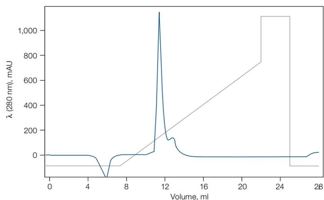
**Fig. 2. PPAR $\gamma$ -LBD purification using 1 ml Enrich Q anion exchange column on NGC Quest system plus sample pump.** The protein was eluted with a 15 CV linear gradient from 0–70% buffer B.  $\lambda$  (280 nm) (—); %B (—). **Note:** Buffer B is the same as Buffer D described in Materials and Methods.
