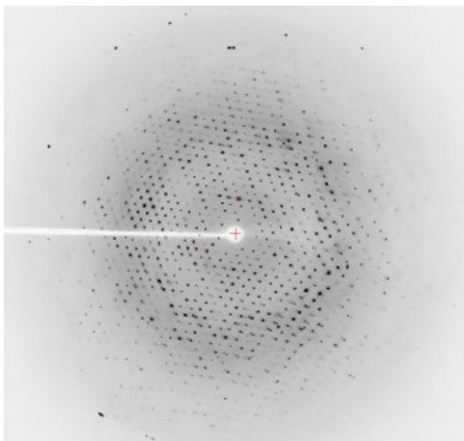
**Fig. 6. Representative diffraction pattern of PPAR $\gamma$ -LBD + S1P.** Crystals were mounted and data collected at beamline MX2 of the Australian Synchrotron. Diffraction images of 1 sec intervals were collected and processed to a final resolution of 2.1 Å.
