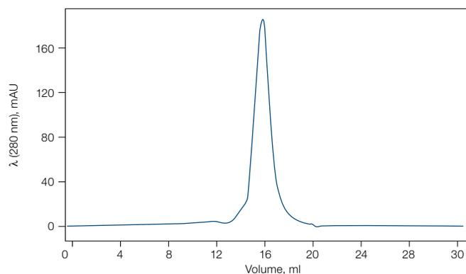
**Fig. 3. PPAR $\gamma$ -LBD purification using 24 ml Enrich SEC 650 size exclusion column on NGC Quest system.** The protein was eluted with a 1 CV isocratic flow of buffer A.  $\lambda$  (280 nm) (—). **Note:** Buffer A is the same as Buffer E described in Materials and Methods.
