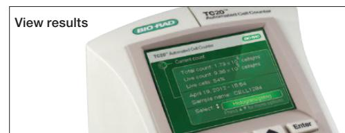
Obtain a total cell count (without trypan blue) or total and live cell counts (with trypan blue) in 30 seconds.
