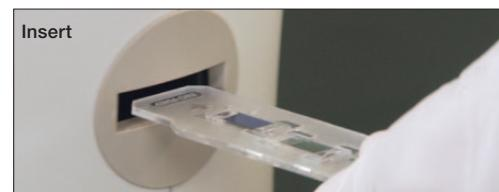
Insert the slide into the TC20 cell counter; counting automatically begins.
