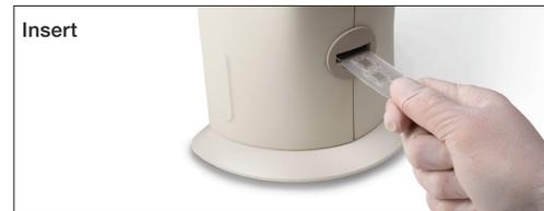
Insert the slide into the TC10 cell counter; counting automatically begins.
