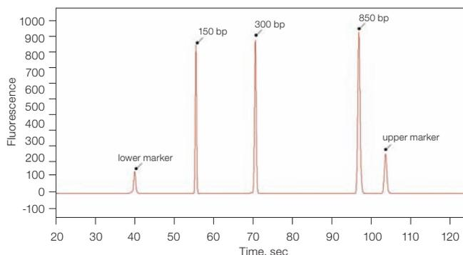
**Fig. 3. Analysis of DNA fragments on the Experion automated electrophoresis system.** Representative electropherogram of three DNA fragments separated on the Experion system using the DNA 1K analysis kit.
