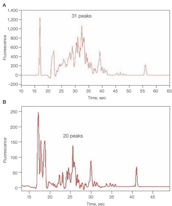
**Fig. 2. Resolution of protein separation.** Comparison of electropherograms of an *E. coli* protein lysate. Using the Experion Pro260 analysis kit (A) and the Agilent Protein 230 assay kit (B), the Experion system reveals a larger number of peaks.
