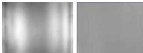
Images of a VersaDoc fluorescent reference plate. Left, VersaDoc image without flat fielding (11% CV); right, VersaDoc image with illumination flat fielding applied (1.1% CV).
