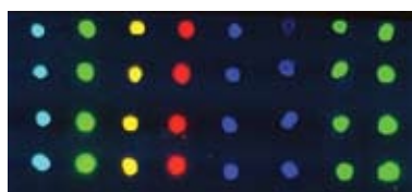
Dot blot of nanoparticles (Invitrogen Corporation and Evident Technologies) imaged on the VersaDoc MP 4000 system.
