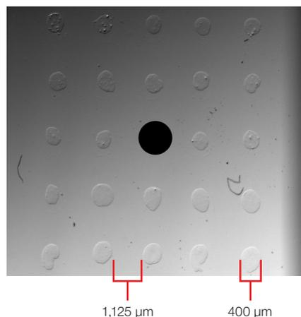
**Fig. 3. Dried spots in one well of a Lab-Tek Chamber Slide.** A total of 25 spots with a distance between each spot of  $\sim 1,125 \mu\text{m}$  and diameters of  $\sim 400 \mu\text{m}$ . The black dot in the center is a mark made by a pen on the external surface of the slide to provide the position for the microscope software.
