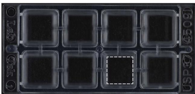
**Fig. 2. 8-well Lab-Tek Chamber Slide.** Each slide is 74  $\times$  22 mm with a thickness of 0.13–0.17 mm and culture area of 0.8  $\text{cm}^2$ . The dashed square presents a well of the Chamber Slide (see Figure 3 for a zoomed spotted version).
