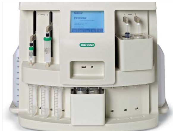
Cooling accessories are shown in place for the sample and fraction collection tubes.
