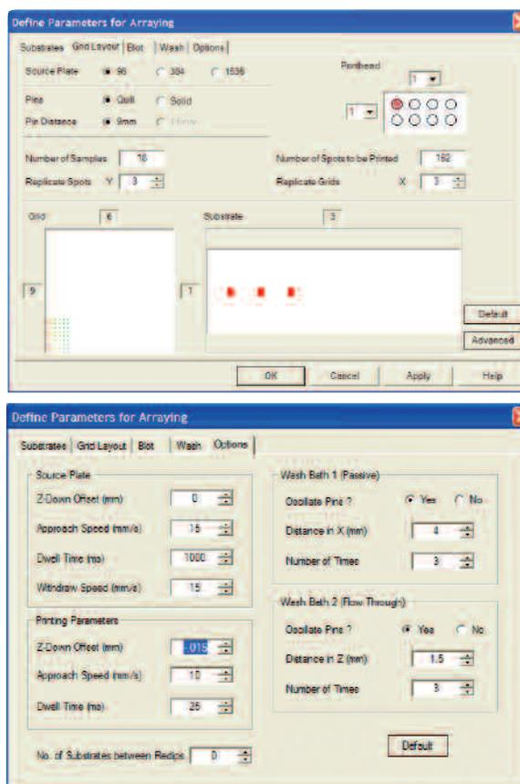
Fig. 2. Arraying program. Upper screen, grid layout window; lower screen, options window.
