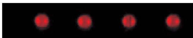
**Fig. 4. Pig snout formed by improper z-height of the solid pins.**
