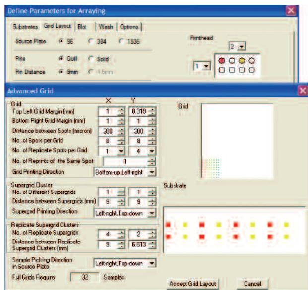
Fig. 1. Parameters for printing onto pad-type slides. Note the margin and supergrid distances.
