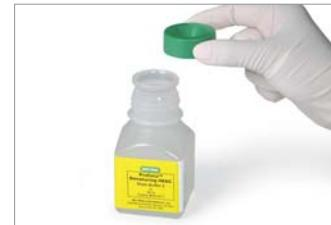
1. The Profinia system includes buffer bottle lids for placement on each buffer bottle to prevent dust and other contaminants from entering the system.
