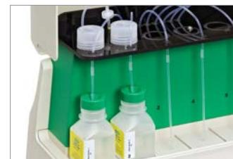
2. The position number on the bottle corresponds to the position number on the Profinia instrument buffer compartment.
