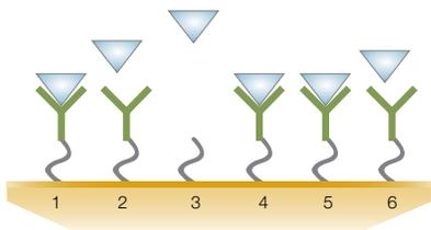
**Fig. 1. Workflow of the ProteOn one-shot kinetics kit.** Step 1, immobilize IL-2 antibody on chip surface. Step 2, inject IL-2 antigen and monitor interaction with immobilized IL-2 antibody. (Channel 3 is a reference channel.)
