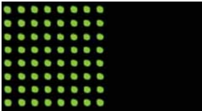
Fig. 1. Image of an 8 x 8 grid generated by one pin for the oligonucleotide carryover assay. Oligonucleotide (left) followed by buffer alone (right) was printed twice on duplicate UltraGAPS slides. Crosslinked oligonucleotide was detected by hybridization to a Cy3-labeled probe. Image is the average result of duplicate slides.
