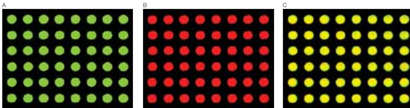
**Fig. 7. Representative image of a grid printed with a single pin for the superimposed image assay using the BioOdyssey Calligrapher.** A, a Cy3-labeled oligonucleotide was first printed; B, a Cy5-labeled oligonucleotide was printed using identical parameters; C, the two images were superimposed.
