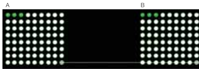
Fig. 5. Representative image of an array printed to assess grid-to-grid regularity. A Cy3-labeled oligonucleotide was printed using parameters for an expected GGX distance of 2.25 mm (indicated by white line).
