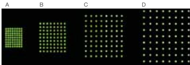
**Fig. 3. Differentially spaced grids (A–D) printed to assess spot-to-spot regularity.** Parameters were defined such that each grid had a distinct CCD for each spot: A, 175  $\mu\text{m}$ ; B, 275  $\mu\text{m}$ ; C, 400  $\mu\text{m}$ ; D, 500  $\mu\text{m}$ .
