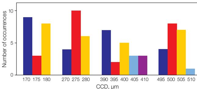
**Fig. 4. Regularity of measured spot-to-spot distances.** CCD between spots in each grid was plotted. Target CCDs for grids were: A, 175  $\mu\text{m}$ ; B, 275  $\mu\text{m}$ ; C, 400  $\mu\text{m}$ ; D, 500  $\mu\text{m}$ .
