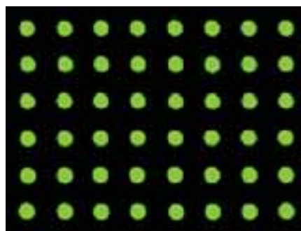
Fig. 2. Representative image of an array printed by the BioOdyssey Calligrapher miniarrayer for the spot morphology assay.
