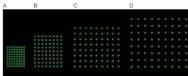
**Fig. 3. Spot-to-spot regularity assay.** Image of an array printed with the VersArray ChipWriter Pro with a Cy3-labeled oligonucleotide. Parameters were defined such that each grid (A, B, C, or D) had a distinct center-to-center spacing of each spot. Center-to-center distances were: A = 175  $\mu\text{m}$ , B = 275  $\mu\text{m}$ , C = 400  $\mu\text{m}$ , D = 500  $\mu\text{m}$ .
