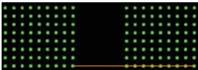
**Fig. 5. Microarray grid-to-grid regularity assay.** A Cy3-labeled oligonucleotide was printed using parameters such that the expected GGX and GGY distances were 5 and 8.62 mm, respectively. Orange line indicates CCD.
