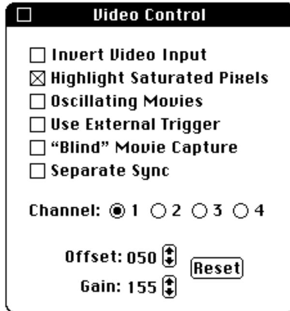
Images acquired using a frame grabber card are inverted if *Invert Video Input* is checked.
