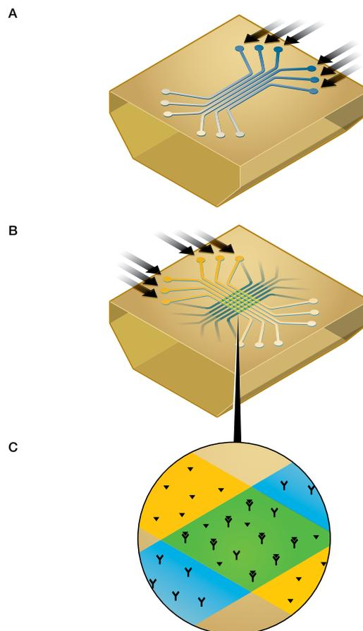
**Fig. 1. Generation of the 6 x 6 ligand-analyte interaction array.** **A**, six ligands are immobilized in six parallel ligand channels; **B**, six analyte samples are injected into six analyte channels orthogonal to the six ligand channels; **C**, detail of a single ligand-analyte interaction spot (green) showing the positions of the two interspot references (yellow).
