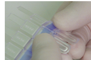
Break off one plastic plug from the casing.
