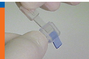
Use spatula to push plug out of plastic casing onto your gel.
